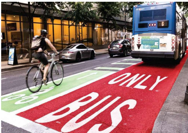
Fig. 2.2: An example of a Kerbside bus lane
